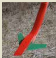
Standard reversible point in combination with 32cm wing share for shallow working.
